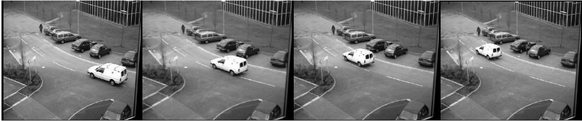
Figure 1: Frames of the sequence that were used to compute the background model. In total 51 frames were used to compute the model.
